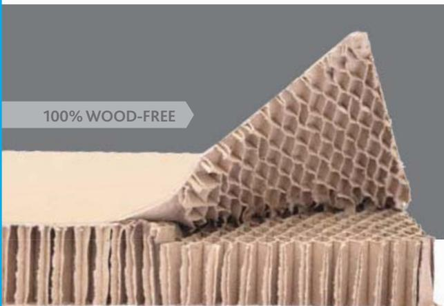
Honeycomb paperboard is an incredibly rigid, yet lightweight paperboard panel that is produced by laminating layers of thick paper onto a paper honeycomb core, resulting in a sandwich-like structure with unsurpassed crush resistance and rigidity.
